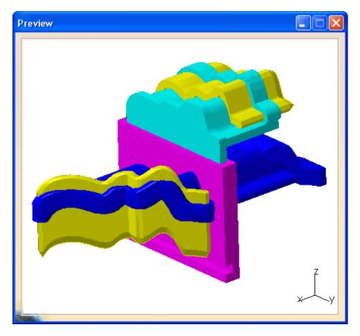
**Select** *Save* **in the window.** A *Save As* window appears. You can save the swept volume as a cgr, wrl, model or stl file. A cgr is a computer graphic representation, a wrl is a VRML file for web viewing, a model file is a V4 file type and an stl is for stereolithography.
