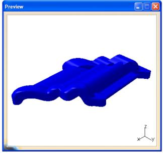
Turn on the Filter Positions with a Filtering precision of 0.005 and select Preview. The preview does not look that much different but it is comprised of fewer triangles and it filtered a majority of the positions.
