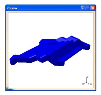
Change the *Filtering precision* back to 0.005, turn on the *Apply Wrapping* option using the default values and select *Preview*. This is like taking a plastic sheet and wrapping the volume with it. Notice that the wrapping reduced the number of triangles.
